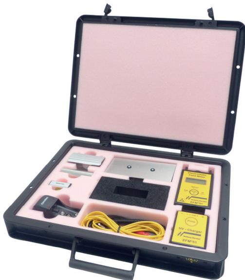
Verification Kit for measuring electrostatic fields and electrostatic charges, as well as the body voltage of a person while performing the walking test. Additionally the decay time and the offset voltage of ionizers can be measured.
