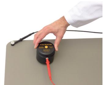
application example: measurement with concentric ring probe
