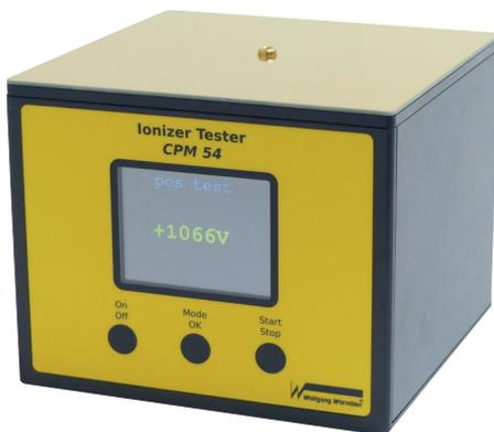
The Ionizer Tester CPM54 is a measuring device for measuring the discharge time and offset voltage of ionizers acc. to the standard, as well as for the measurement of the body voltage (walking test). It supports fully automatic testing of positive and negative discharge as well as offset voltage.
