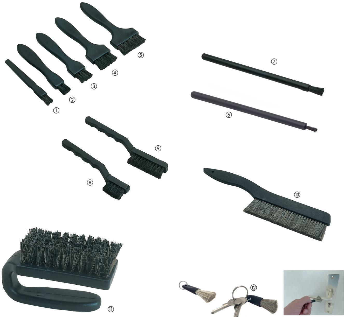
Our range of conductive brushes allows thorough cleaning of ESD sensitive assemblies without the danger of high charges generated by conventional brushes. They consist of a conductive plastic handle and bristles made of highly conductive fibers which will dissipate any charges by corona discharge, due to their small diameter. Natural hair is mixed with the conductive fibers to provide the desired stiffness. Includes the ESD Symbol.
