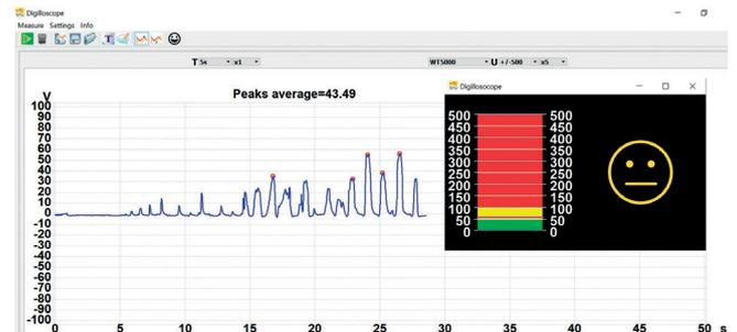
Body voltage measurement test set-up. The software „Digilloscope“ can mark the five highest peaks automatically and calculates the average value.
