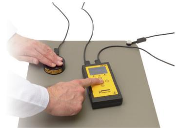
Verification Kit for measuring conductive and dissipative surfaces.
