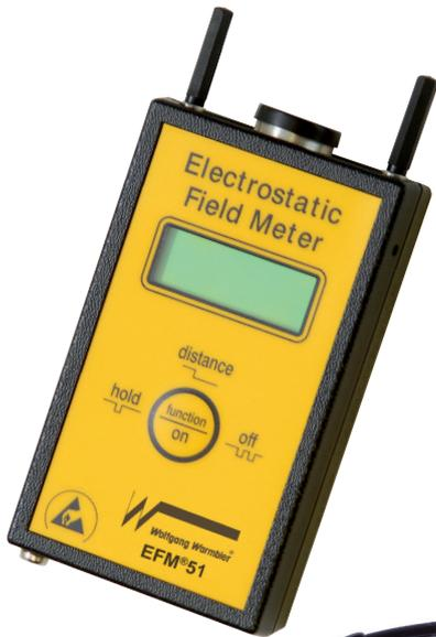
Handheld, portable, digital electrostatic field meter, detects and measures electrostatic fields. The electrostatic field strength value (V/m) will be automatically translated to the electrostatic potential (V) according to the preset distance. An additional field strength mode is also available.
