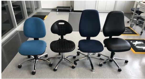
Figure 7: ESD chairs used for “Chair Walking Test” (A to D from left to right)
