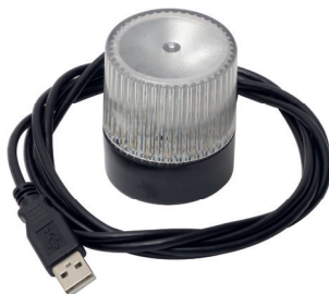
7100.PGT120.TEST.13 USB HID Visual Signal
